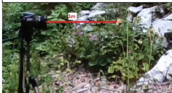
Figure 3 – Nikon D5200 with Sigma 10-20mm lens set up 1m away from specimen.
